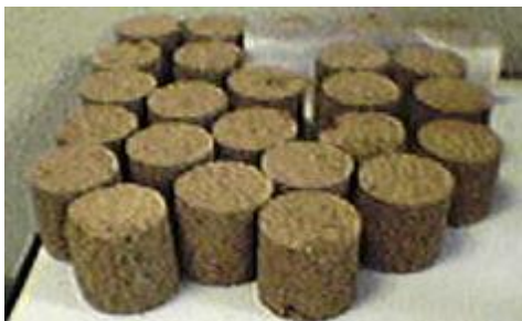
Fig. 1. Samples of test specimens for green compressive strength, permeability and shatter index.
